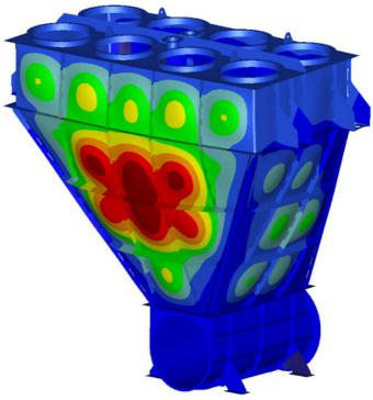
A separate series of analyses was also performed in support of design development of the hopper outlet flange, which incorporated an unusual double seal arrangement not catered for by standard design code rules.
